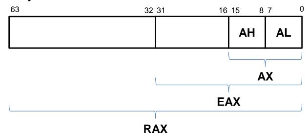
This is a single 64 Bit register – only subparts with different names!
